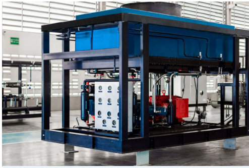
Natural gas compressor
